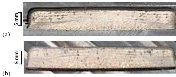
Fig. 10: Image from the thin wall built with (a) monitoring only; and (b) active closed-loop
