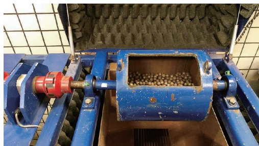
Fig. 1 8"×10" jar mill equipped with a torque sensor.
