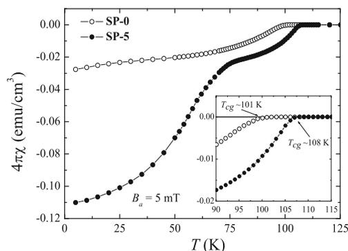
**Fig. 3** Temperature dependence of magnetization measured in bulk samples under an applied magnetic field of 5 mT. Only the ZFC branches are displayed in the figure. Changes in  $T_{cg}$  are seen after the post-annealing heat treatment performed at 750 °C for 5 min
