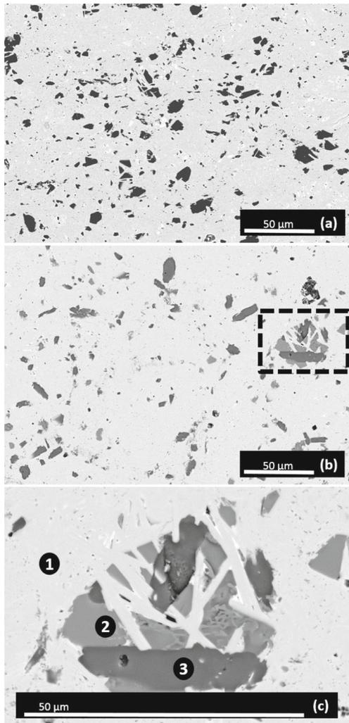
**Fig. 1** SEM images (*back scattered electrons images*) **a** sample SP-0, **b** SP-5 sample, and **c** expanded view of SP-5 sample showing details of the microstructure in which crystal phases identified by different *gray shades* may be observed. The image correspond to the surface of the sample perpendicular to the applied pressure direction. The chemical compositions of points 2 and 3 were found to be very similar
