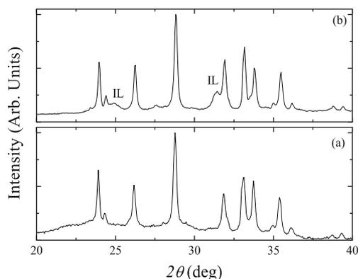
**Fig. 2** XRD patterns of pellet samples of **a** SP-0, and **b** SP-5. The extra peaks belonging to the infinite-layer phase (marked as IL) appears after the post-annealing treatment
