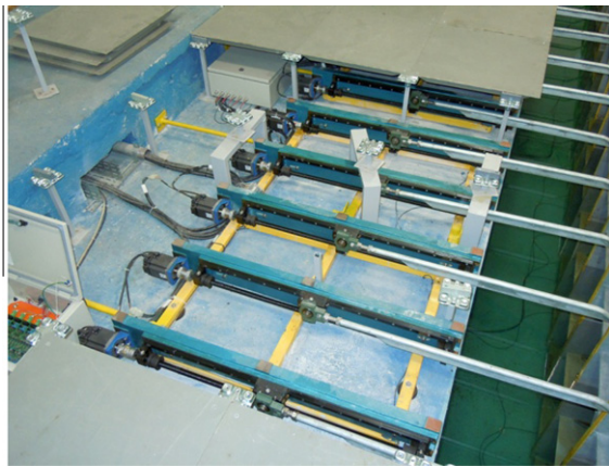
(a) Frame with 5 linear actuators mounted in the wave tank.
