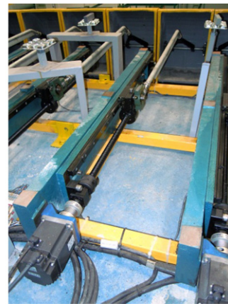
(b) Detail of one actuator using ball screw and linear guide.
