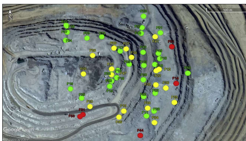
Fig. 6. Boreholes locations, in the open pit mine located at Catalão-GO in Brazil, classified regarding the radiological hazard indices.
