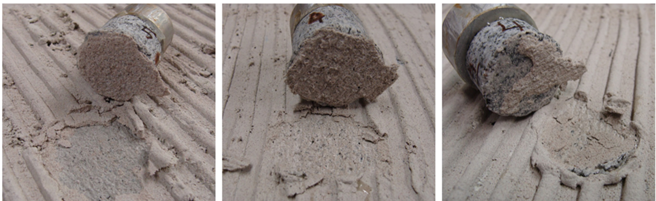
Fig. 6 – Partial view of substrates with application of “M2” mortars, after TBS tests of CA monzogranite specimens with 30 mm diameter (LEFT, CENTER) Detail showing failure in the mortar-standard substrate interface (tests at temperatures of 23 °C and 40 °C, respectively) (RIGHT) Detail showing mixed failure (part in mortar and part in substrate) common in tests at temperatures of 60 °C.
