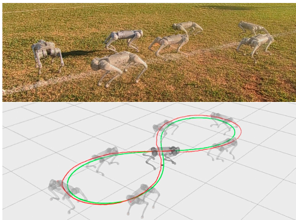
Figure 25. Real robot following lemniscate curve with proposed body control and Unitree motion control. Reference trajectory in green and the robot's executed trajectory in red.
