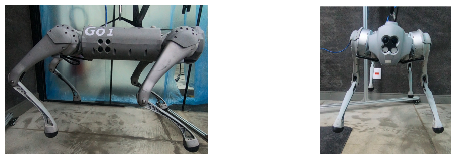
Figure 18. Tests with the physical robot suspended in the air.
