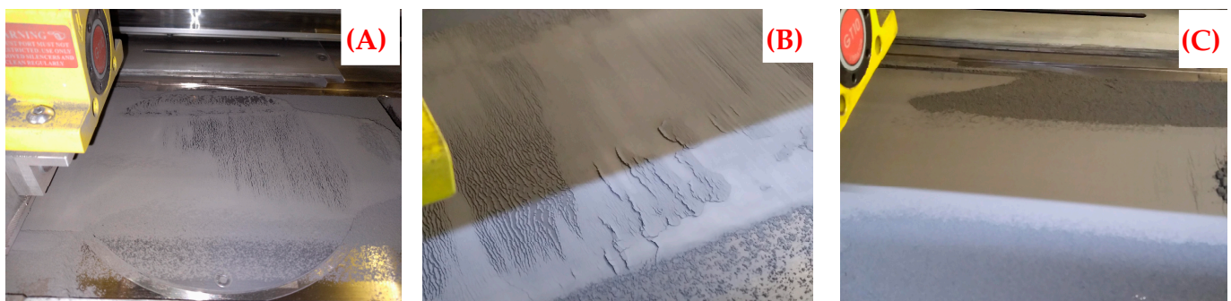
Figure 10. Flow rate and spreadability behavior of mixtures in the powder bed, as a function of the system pressure or device vibration frequency: (A) lack of adhesion between particulates; (B) craters and “alligator shell” and (C) uniform, homogeneous, and continuous flow from the central part of the powder bed.
