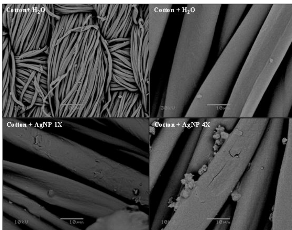
Figure 3. Scanning electron microscopy of the cotton fabrics without impregnation (cotton + \text{H}_2\text{O} ) and impregnated with AgNPs by one and four times. Cotton + \text{H}_2\text{O} (100 and 10 \mu\text{m} ); cotton + AgNPs 1x (10 \mu\text{m} ); cotton + AgNPs 4x (10 \mu\text{m} ).
