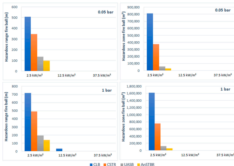
Figure 4. Hazardous zone and range for fireball heat flux.
