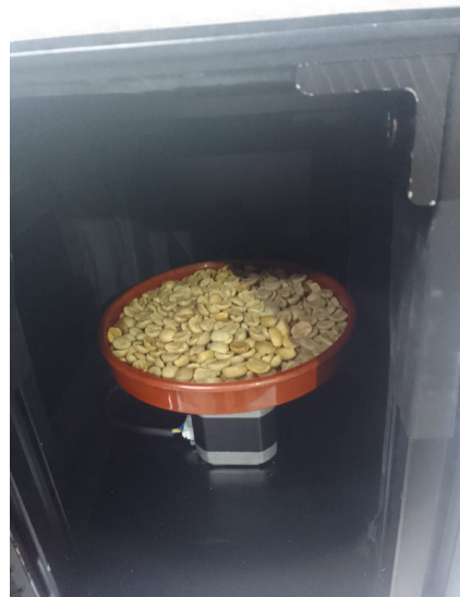
Figure 3. Robusta coffee samples inserted in the RGB Analysis System.
