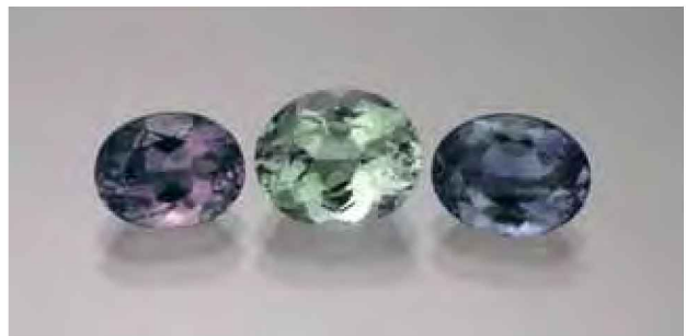
Figure 40. These samples show the coloration of the Montezuma mine quartz as untreated amethyst (left, 2.40 ct), heated green quartz (center, 3.54 ct), and heated and irradiated violet quartz (right, 2.37 ct). Gift of Henrique Fernandes and Gabriel Freitas, Pinkstone International, Governador Valadares, Brazil; GIA Collection nos. 36697–36699. Photo by Robert Weldon.
