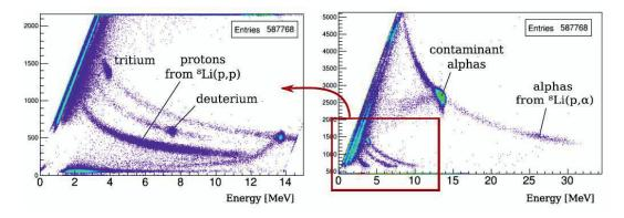
Figure 4. Bidimensional energy spectra obtained using a Si telescope at  $\Theta_{lab}=10^{\circ}$ , in the large chamber after the second solenoid, with the secondary beams focused on a  $[CH_2]_n$  target. The spectrum on the left is a zoom of the spectrum on the right.
