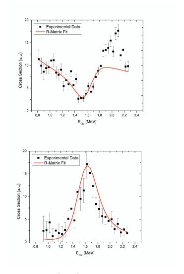
**Figure 5.** The excitation function of the  ${}^8\text{Li}(p,p){}^8\text{Li}$  reaction, together with a fit by the R-matrix calculation is shown on the top. On the bottom is the excitation function of the  ${}^8\text{Li}(p,\alpha){}^5\text{He}$  reaction, together with a fit by the R-matrix calculation.
