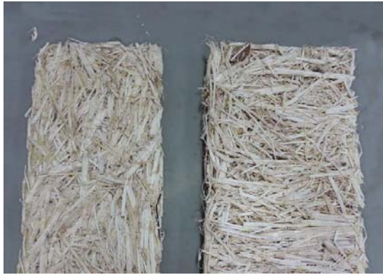
Figure 7: sugar cane bagasse and castor oil resin boards before attachment
