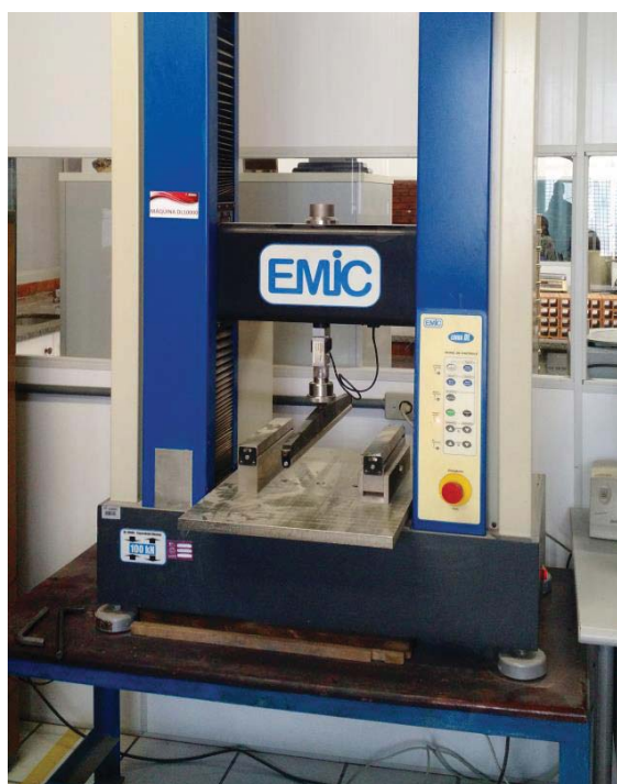
Figure 17: EMIC's DL10000, with a proper fixture set installed
