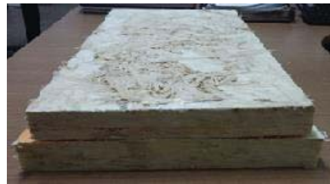
Figure 11: sugarcane bagasse and polyurethane foam filler component
