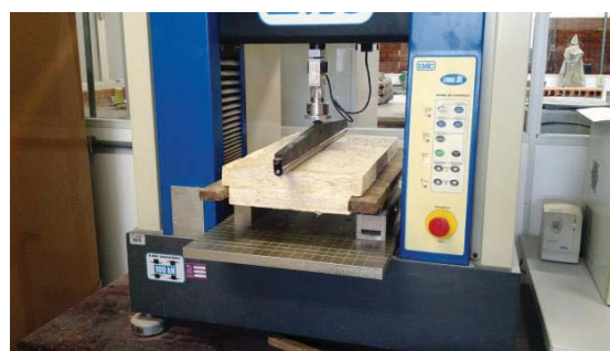
Figure 20: breaking load test setup (second prototype)
