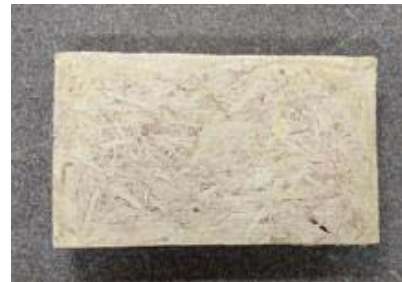
Figure 12: sugarcane bagasse and polyurethane foam filler component
