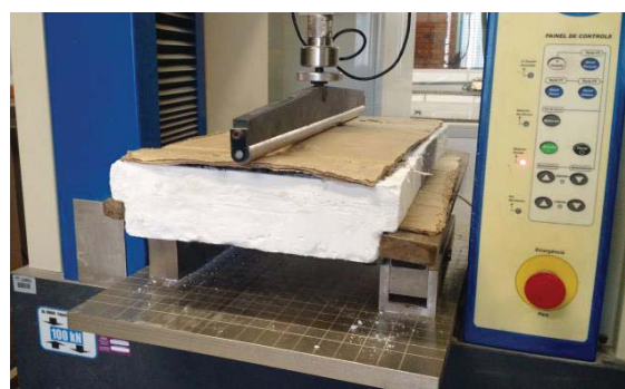
Figure 18: Breaking load test setup (first prototype)
