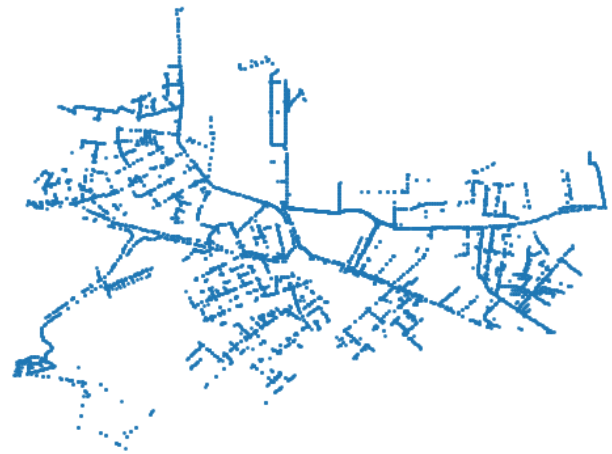
Figure 1. Graph representation of a Brazilian Electric Power Distribution System, composed of 3536 nodes, 3254 edges.
