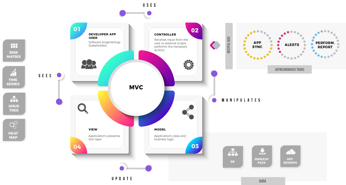
Figure 29. MVC architecture of the MApp-IDEA tool
