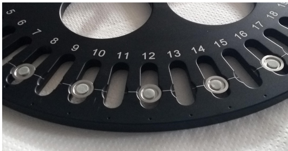
Figure 1: Alexandrite – polymer pellets arranged on stainless steel sample holders.
