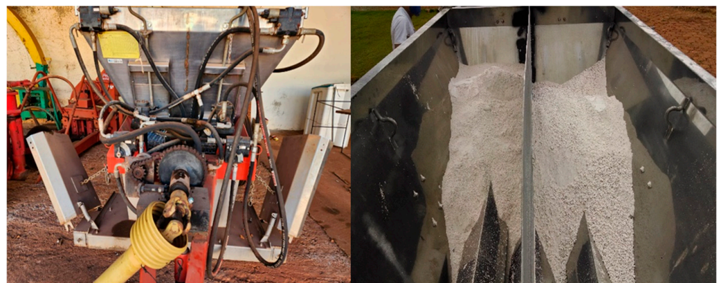
Figure 1. Fertilizer spreader variable-rate application system and machine reservoir adaptation.
