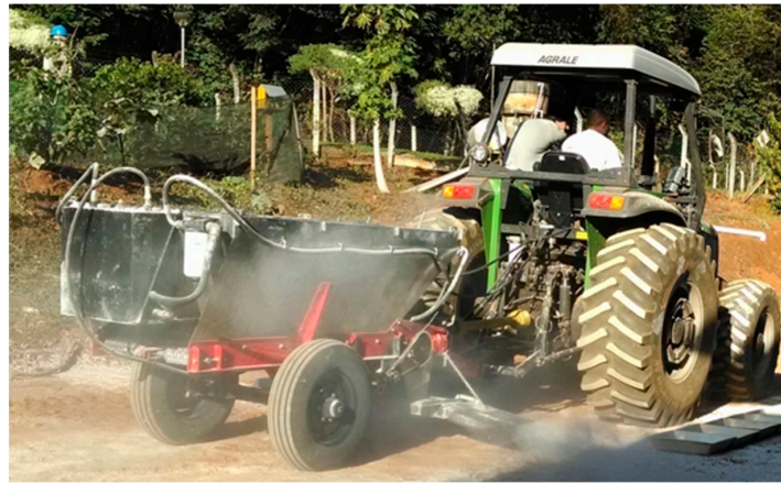
Figure 2. Mechanized tractor and fertilizer spreader set used in the test.
