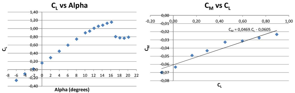
Figure 11. Wing alone - aerodynamic coefficients.
