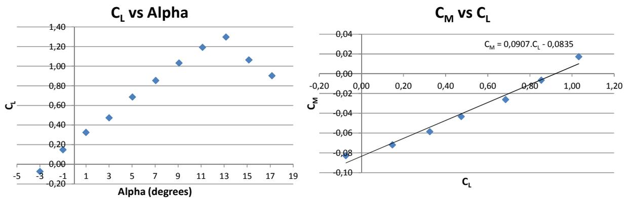
Figure 16. Configuration 5 - aerodynamic coefficients.
