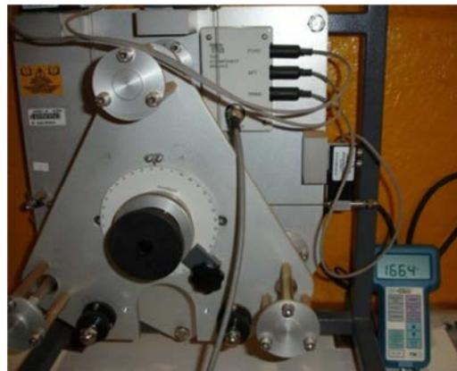
Figure 9. Aerodynamic balance and digital manometer.
