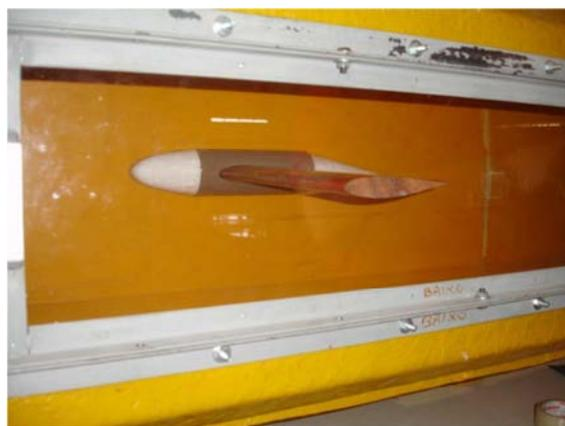
Figure 7. Model at wind tunnel test section.
