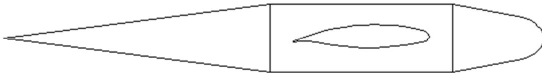
Figure 4. Configuration 4: short forward and extended rear fuselage segments, total length of 0.590 m (scale 1:4).
