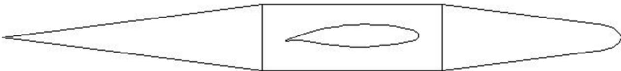
Figure 1. Configuration 1: extended forward and rear fuselage segments, total length of 0.690 m (scale 1:4).
