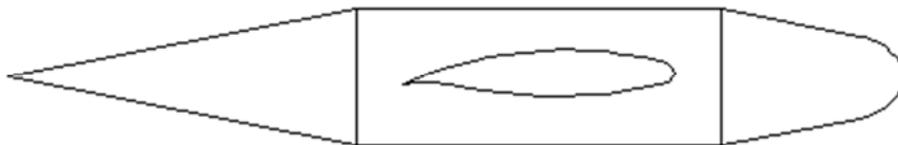
Figure 5. Configuration 5: short forward and rear fuselage segments, total length of 0.490 m (scale 1:4).
