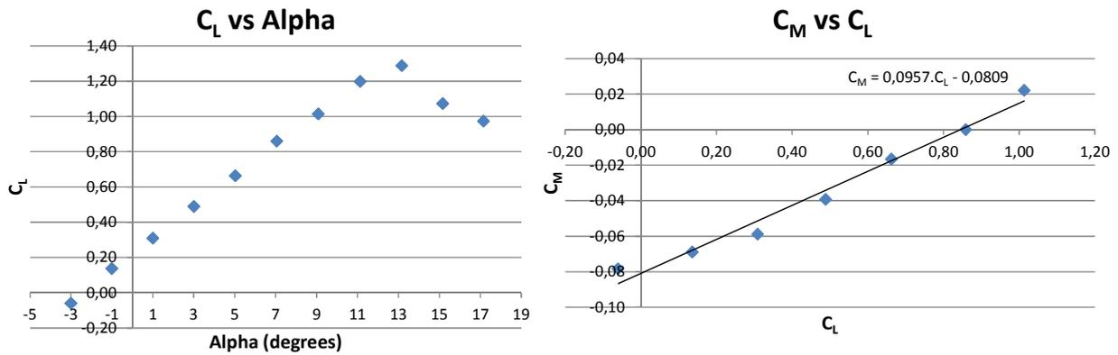
Figure 15. Configuration 4 - aerodynamic coefficients.
