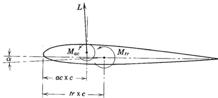
Figure 8. Geometry and parameters used for calculating the wing aerodynamic center position for a wind tunnel test (Barlow, *et al.*, 1999).
