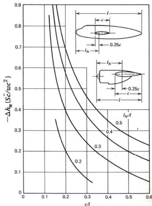
Figure 10. Fuselage and nacelle effects on neutral point position (Etkin and Reid, 1996).
