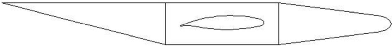
Figure 3. Configuration 3: extended forward and asymmetrical rear fuselage segments, total length of 0.690 m (scale 1:4).
