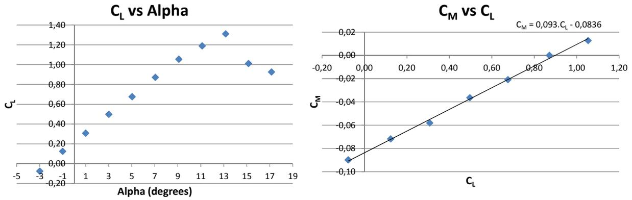
Figure 14. Configuration 3 - aerodynamic coefficients.
