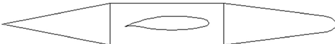
Figure 2. Configuration 2: extended forward and short rear fuselage segments, total length of 0.590 m (scale 1:4).
