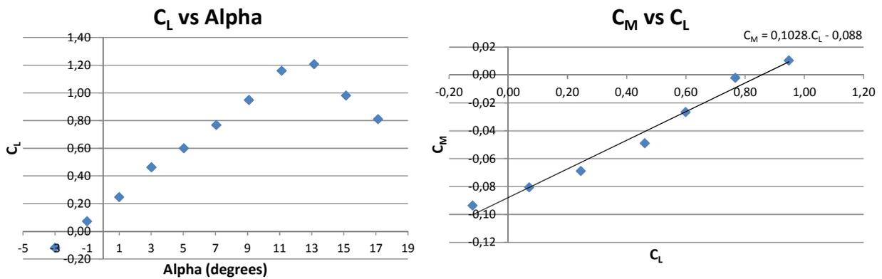
Figure 12. Configuration 1 - aerodynamic coefficients.
