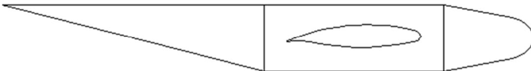
Figure 6. Configuration 6: short forward and asymmetrical rear fuselage segments, total length of 0.590 m (scale 1:4).
