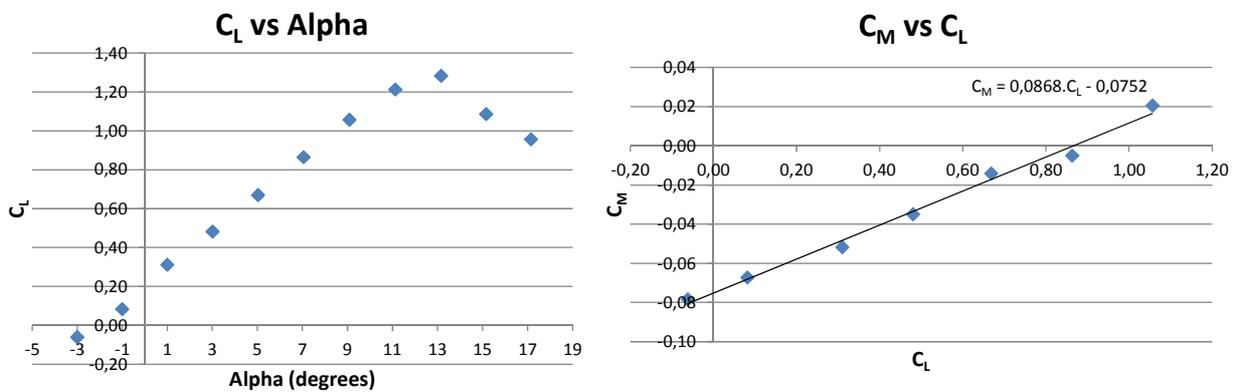
Figure 13. Configuration 2 - aerodynamic coefficients.
