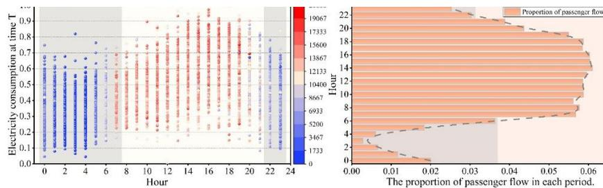
Figure 3. Correspondence between passenger flow and electricity consumption at time T, with (a) hourly passenger flow and electricity consumption and (b) percentage of hourly passenger flow.
