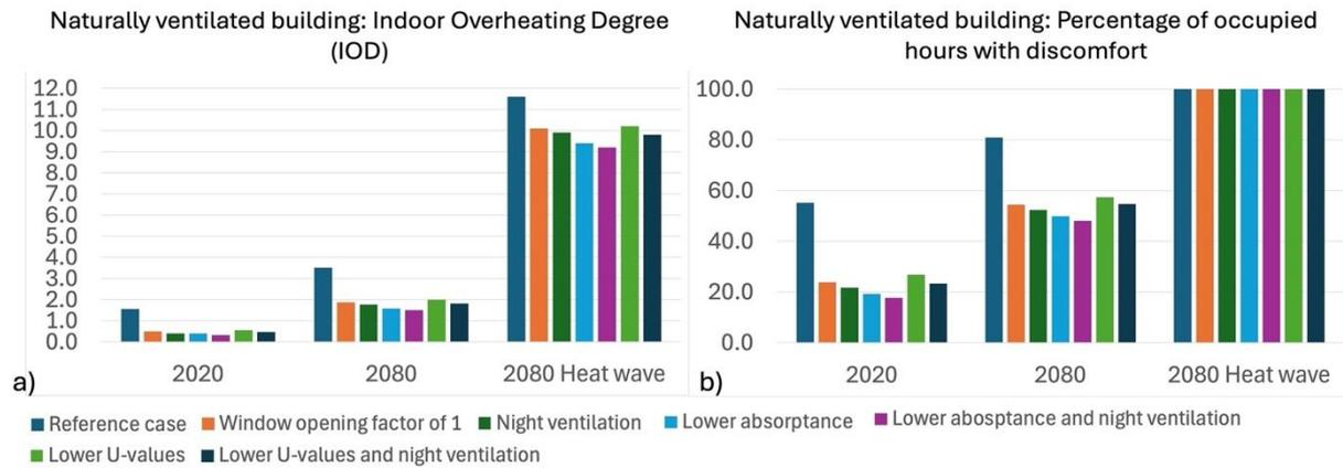
Figure 1. Naturally ventilated cases indicators a) IOD and b) percentage of occupied hours with discomfort.
