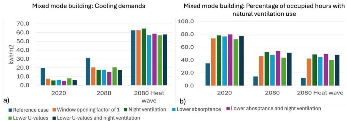
Figure 2. Mixed mode cases indicators a) cooling demands and b) percentage of use of natural ventilation.
