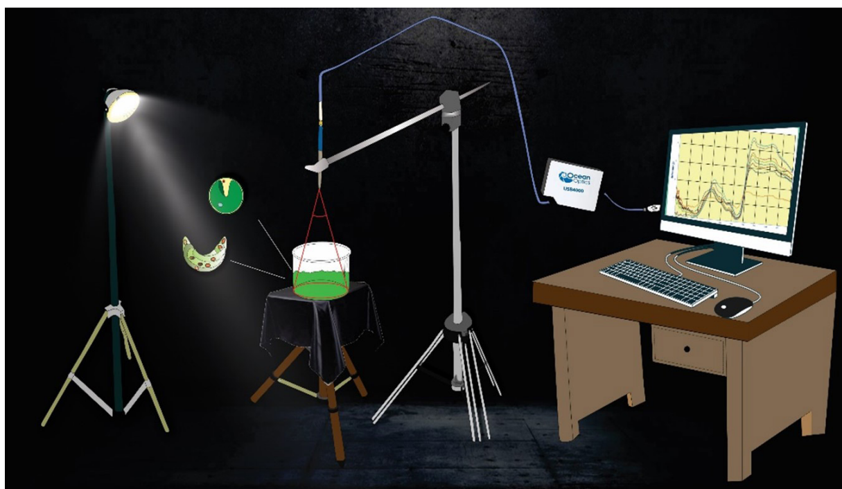
Figure 3. Schematic of the use of the Ocean Optics USB 4000 Spectroradiometer in the laboratory to measure the energy reflected by the microalgae Chlorella vulgaris and Raphidocelis subcapitata when they interact with the electromagnetic radiation artificially generated by a 1000-watt tungsten lamp. The results are presented in graphs with the wavelengths on the X axis and the reflectance percentages on the Y axis.
