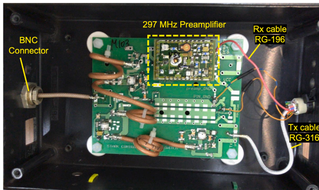
Fig. 2. 300 MHz TR Switch with BNC connector used to interface the flat solenoid coil with the 7T MRI scanner. Everything was assembled inside a plastic box, which can be used as an interface box for different designs of homebuilt RF coils.
