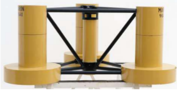
FIGURE 2: Picture of the model-scale floater analyzed in the DeepCwind project. Extracted from [16].
