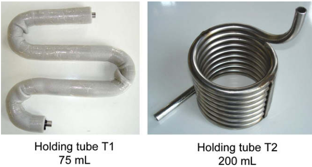
Fig. 4. Holding tubes T1 and T2 of the FT-43 laboratory plate pasteurizer (thermal insulation of T2 was removed for better view).
