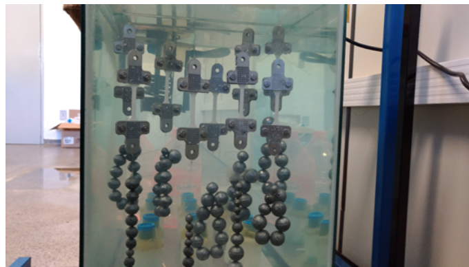
Figure 7. Degradation experiment of biodegradable polymers regarding different stress fields [36].
