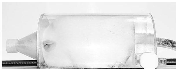
Figure 1. Acrylic cylinder for the ventilatory muscle training of rats.
