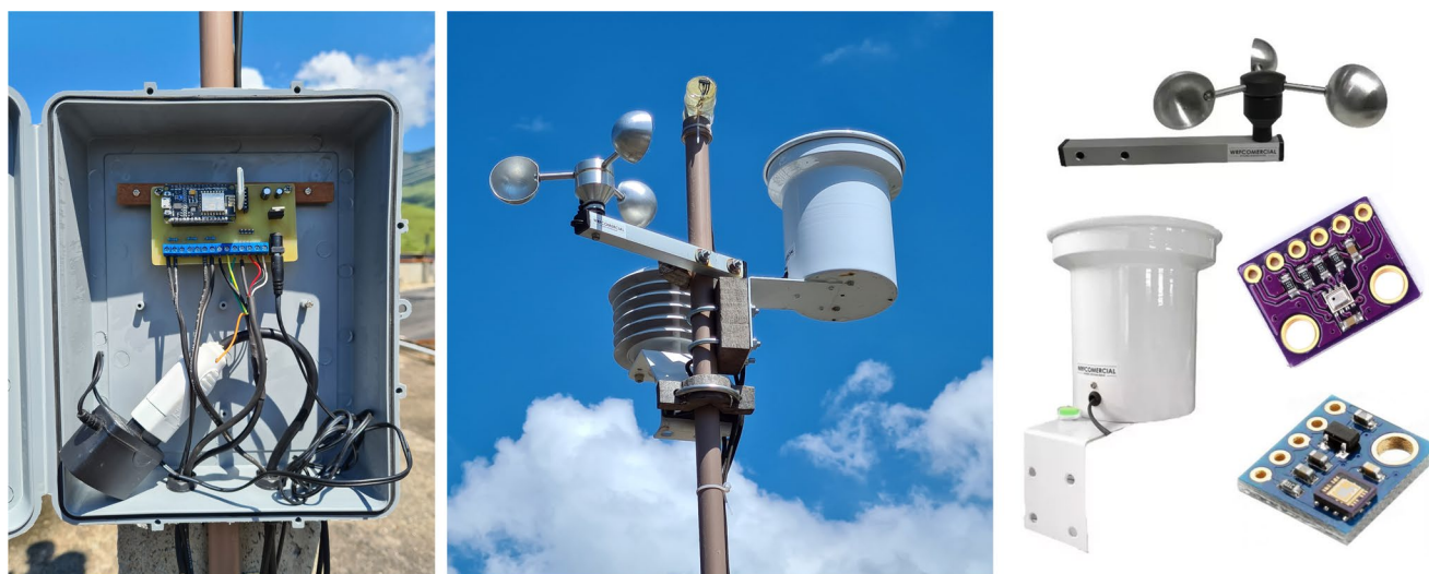
Fig. 7 Developed weather station IoT, including: datalogger mounting box, sensor bar on the station tripod and uses sensor elements (left to right)
