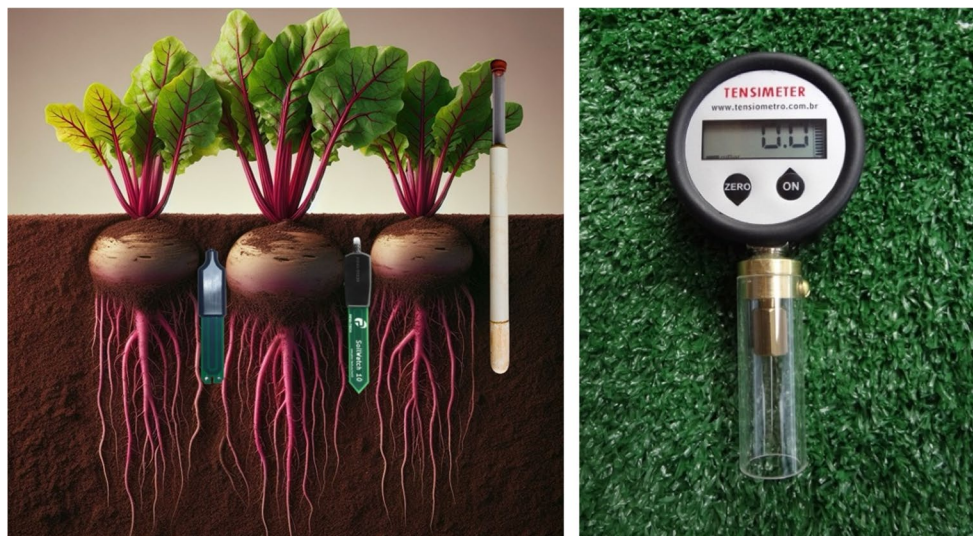
Fig. 3 A - Digital tensiometer used for reading the tensiometer; B - Moisture sensor elements installed next to beet, being VCS, SoilWatch and tensiometer (left to right)
