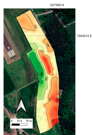
Figure 2. Altimetry map of the experimental field, with respective contour lines. The higher portions are colored in green tones and the lower portions in red tones.
