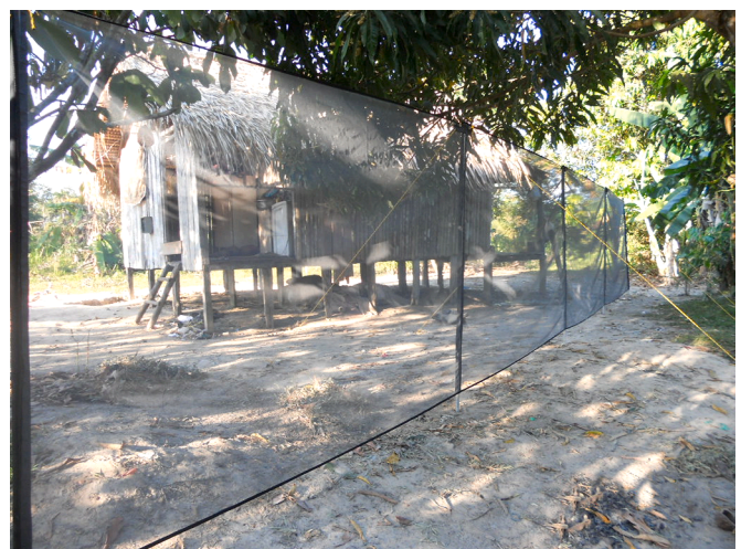
Fig. 1. Barrier made in gray fiberglass screen. Every 3 meters, a 2-meter aluminum tube was attached to keep the screen stretched and without folds that could hinder the collection of the resting mosquitoes.
