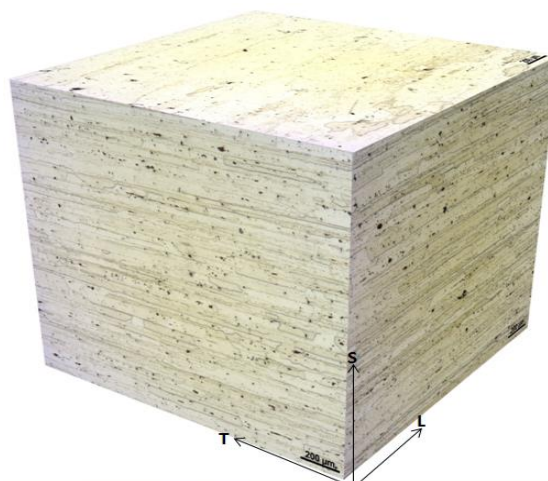
Figure 2 – 3D grain morphology.
