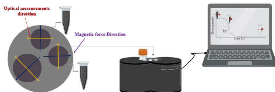
Figure 1. A schematic top view of the magnetic separation setup, which has three cavities with a volume of 2 mL for two tubes and 15 mL for the third tube. The red arrows indicate the movement of MNPs under the influence of magnetic field gradients.
