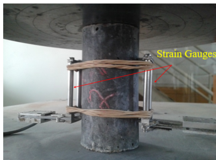
Figure 2. Cyclic test setup.
