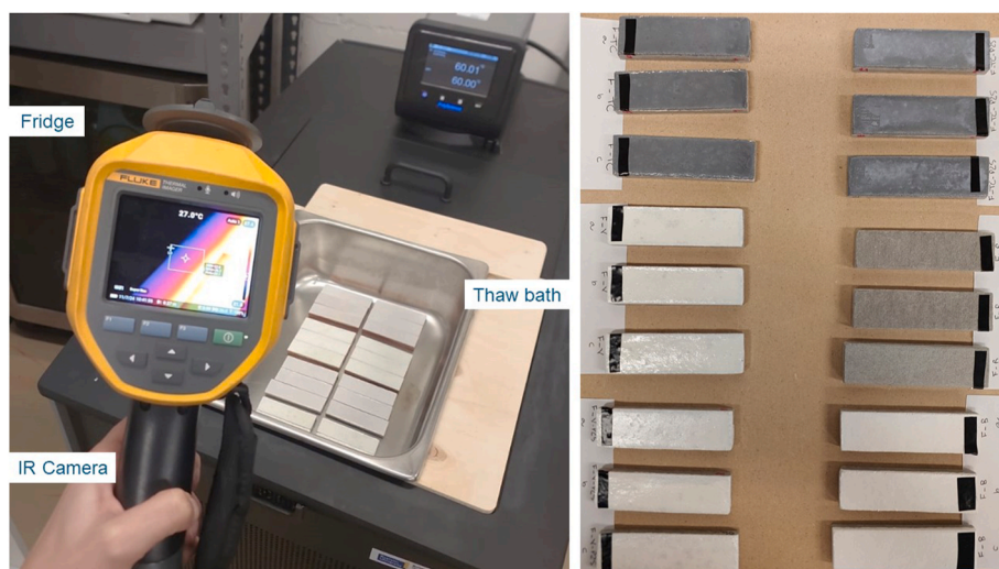
Fig. 3. a) Thermal emissivity temperature control system; b) Black tape applied.
