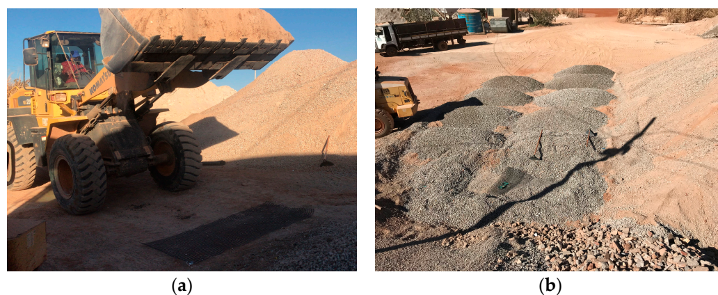
Figure 2. Experimental test to simulate the damage of geosynthetics: (a) positioning of the wheel loader for launching the backfill from 2.0 m height; and (b) configuration after the dropping process of some scenarios and the start of the geogrids' exhumation.
