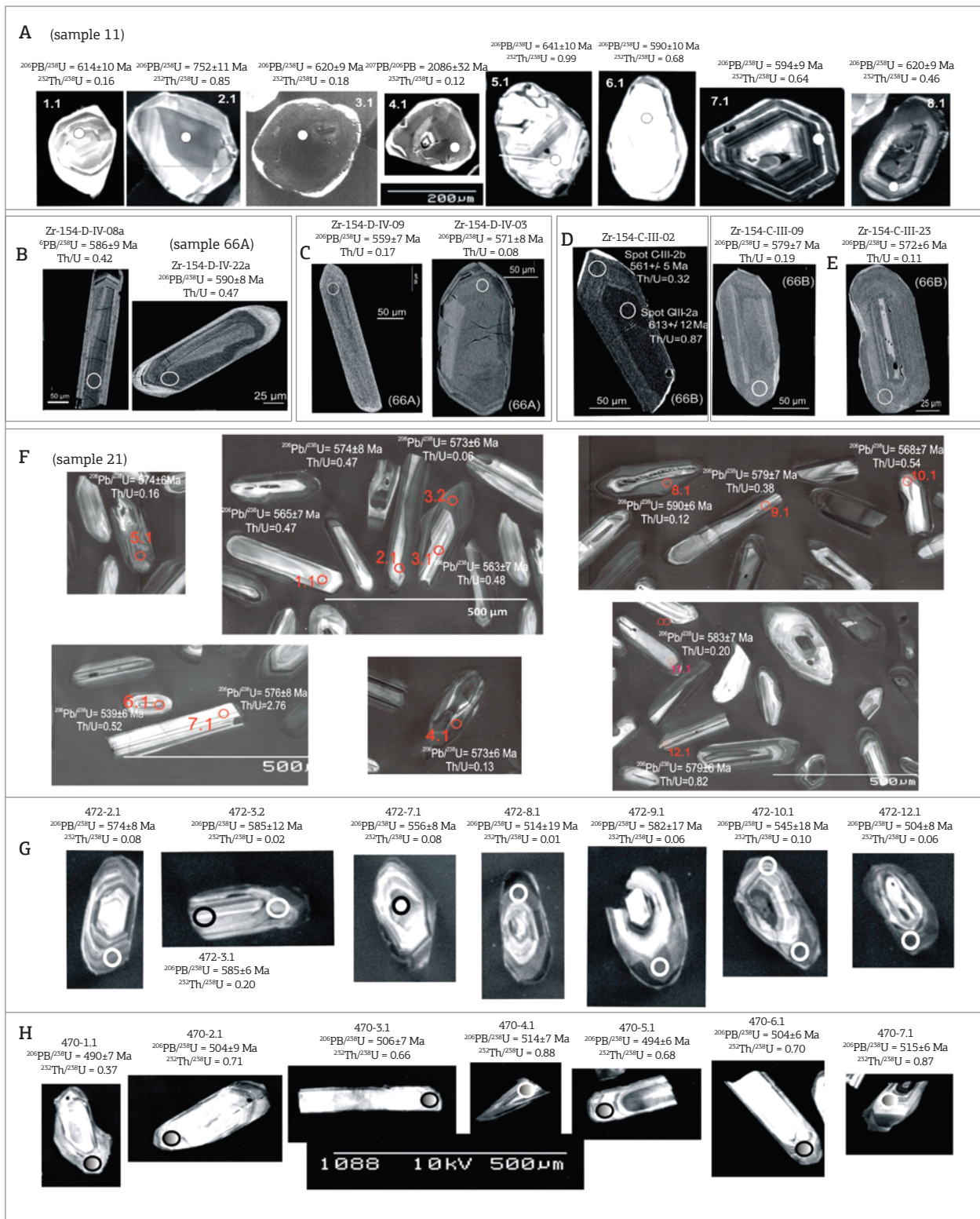
Figure 15. Selected zircon images (CL, cathodoluminescence; EBS, electron backscattering). (A) detrital zircon grains from Nova Venécia paragneisses (sample 11, CL); (B) igneous and (C) metamorphic crystals from an Ataléia foliated granite (sample 66A, Fig. 17D, EBS); (D) igneous core and metamorphic rim in a zircon crystal from Carlos Chagas foliated granite (sample 66B, Fig. 17C), and (E) two metamorphic grains from 66B sample (EBS); (F) igneous crystals from a non-deformed isotropic Carlos Chagas granite (sample 21, CL); (G) metamorphic zircon grains from the ultramylonitic Carlos Chagas granite (sample 472); (H) zircon crystals from the Barra do São Francisco charnockite (sample 470, CL).
