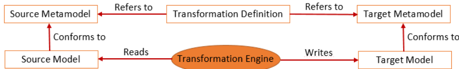
Fig. 3 A simple Model-To-Model transformation scheme. [4]
