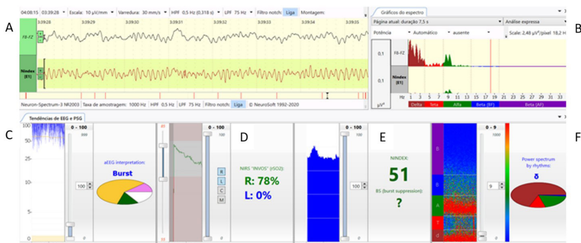
Fig. 1 - Parameters exhibited vertically in a 10-minute trend window: A) continuous electroencephalogram; B) spectral graphic (spectrum); C) amplitude-integrated electroencephalogram (aEEG); D) rScO_2 ; E) NINDEX and F) -spectrogram, recorded at Fz-F8 channel from a two-years old patient undergoing ventricular septal defect repair.
