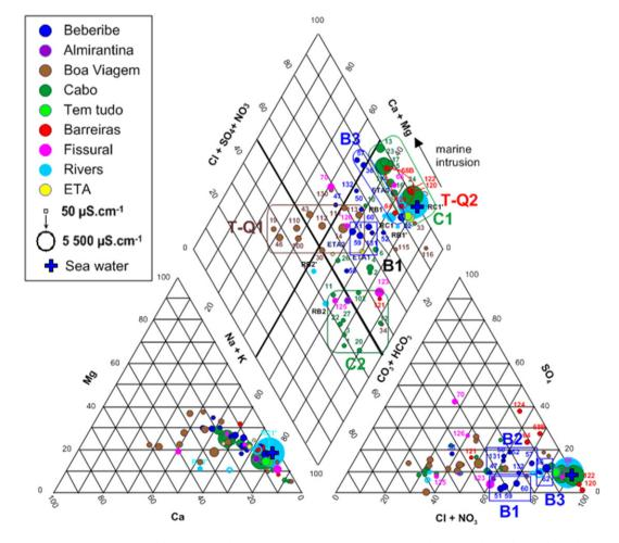
Fig. 3. Piper diagram with groundwater data. Groups of dots are indicated according to their geochemical proprieties. Bx refers to Beberibe aquifer, Cx refers to the Cabo aquifer and T-Qx to the Tertiary-Quaternary deposits of the Boa Viagem and Barreiras aquifers.
