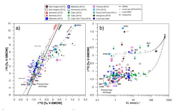
Fig. 5. a)  $\delta^2$ H and  $\delta^{18}$ O isotopes of the water molecule with the LMWL, and b)  $\delta^{18}$ O vs. CI concentrations measured during the sampling campaigns of 2012 and 2013 in rainwater, surface waters, and groundwaters of the RMR in 2012, 2013 and 2014. Dashed lines are mixing lines between seawater and ETAs according to Faure (Faure, 1986).
