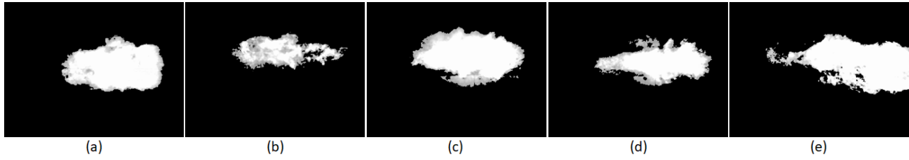
Figure 2 – (a) Stable flame. (b) Unstable flame. (c) Low excess air flame. (d) High excess air flame. (e) Poorly atomized flame
