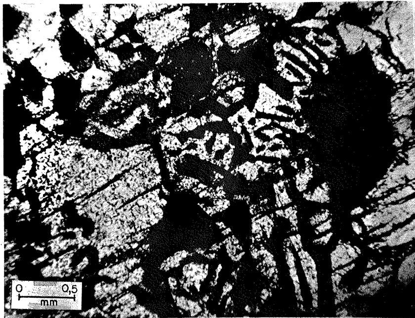
Photomicrograph 1 — In black, sapphirine in symplectitic intergrowth and as granules; bronzite is light-grey and shows good cleavage (crossed nichols).
