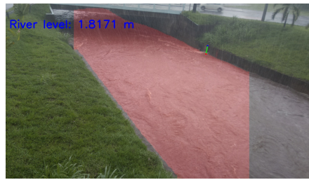
(b) Water level starts to rise. River level is computed as 1.82 meters.
