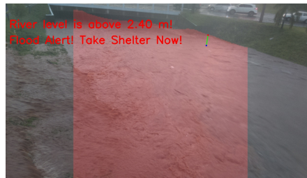
(d) The heavy rain overflows the river. Our system detects that the river has overflowed. The system does not compute the water level once it is above the floodwall.
