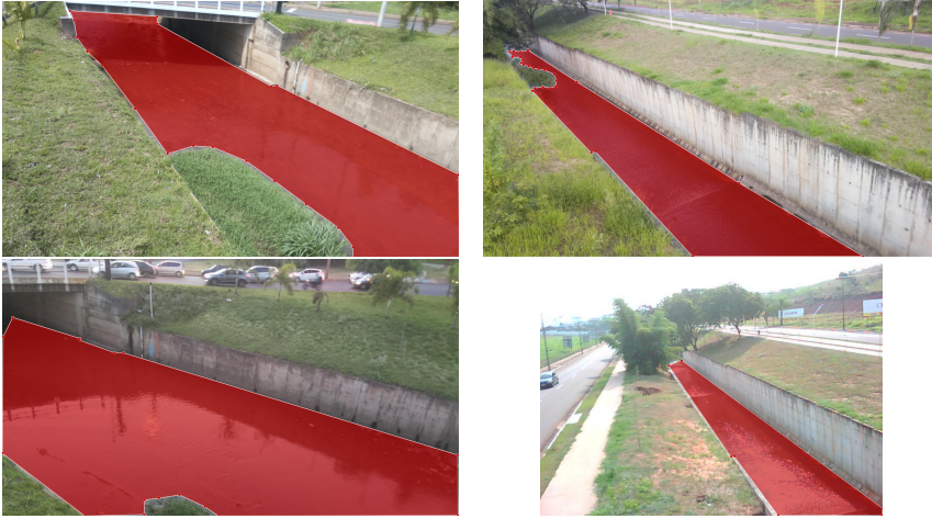
Fig. 5: Examples of manually segmented water surfaces used to train the DeepLabv3 DNN.
