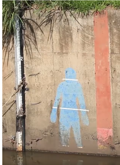
Fig. 11: Ruler installed at river A's bedside. We use this ruler to verify how well our algorithm performs.
