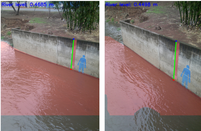
Fig. 8: Water segmentation and water level detection results using images of a single river from different viewpoints.
