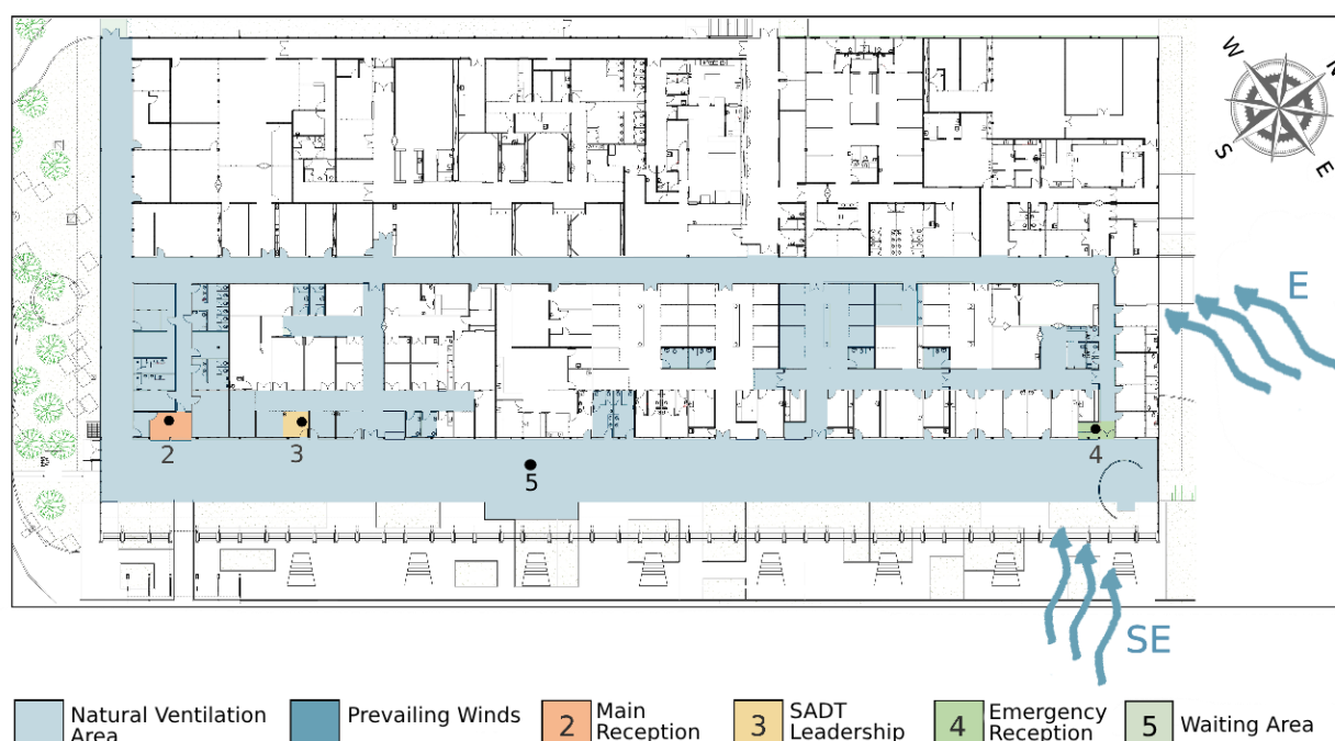
Figure 4 – Thermal zones positioned on the floor plan of Block B of the HU-UFSCar
