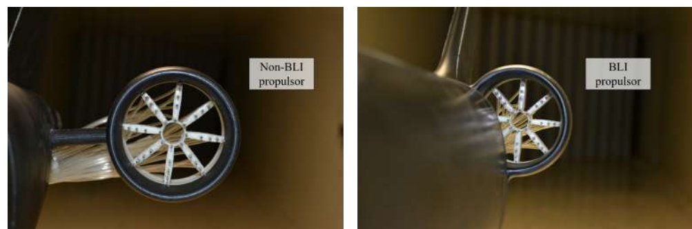
Figure 8. Total pressure rakes installed on the wind-tunnel models.
