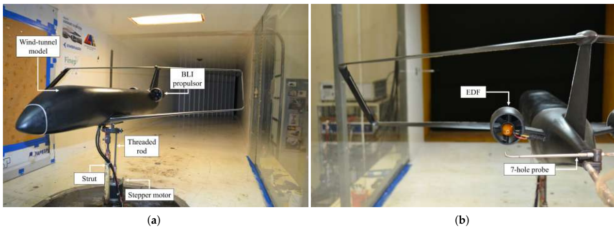
Figure 7. Overview of the wake mapping experiment in the test section. (a) BLI configuration installed in LAE-1. (b) Close-up view of the probe installation for the non-BLI experiments at LAE-1.
