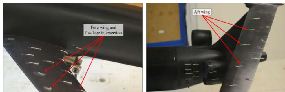
Figure 11. Mini-tuft flow visualization on the wing surfaces at M = 0.089 , Re = 3.02 \times 10^5 , and \alpha = 10^\circ .
