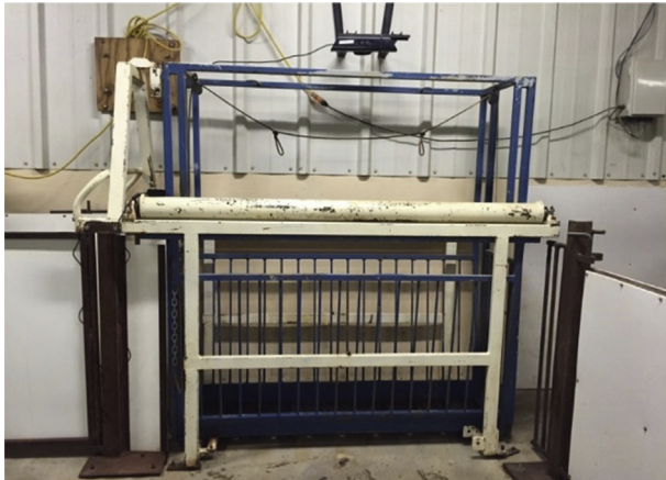
Fig. 1 – Mass and images were captured on individual pigs using a standard pig weighing scale and Kinect® sensor, version 1. The Kinect® sensor was mounted on the wall directly above the centre of the scale.
