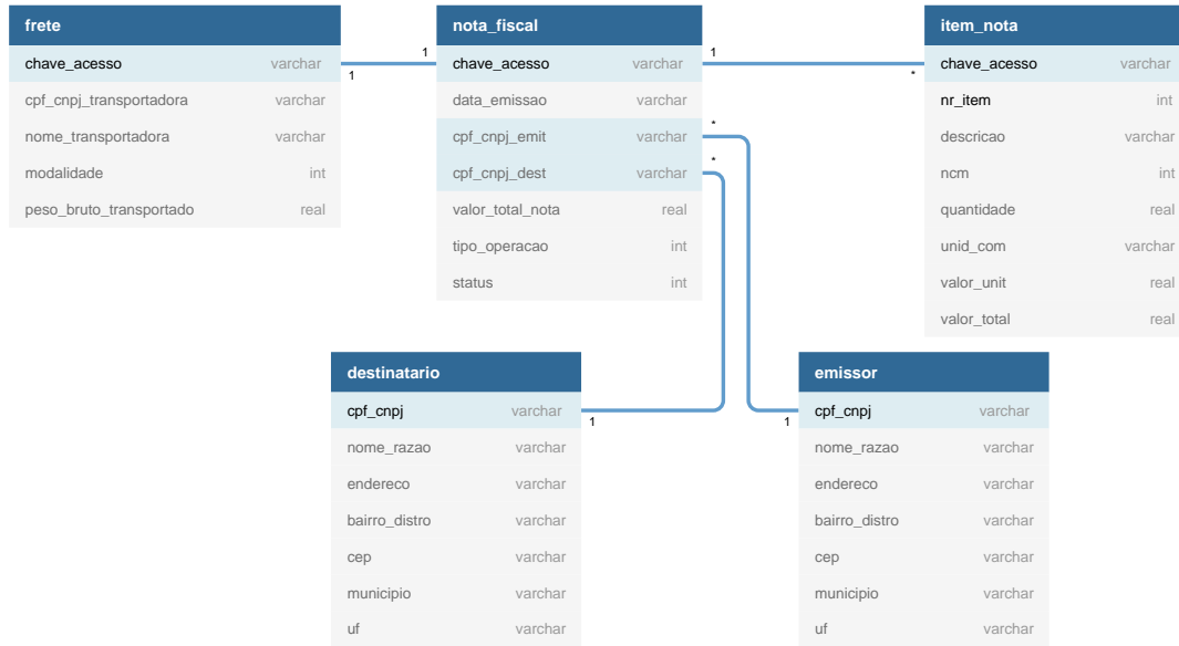
Fig. 2. Basic relational model composed of five tables obtained from XML invoice files.
