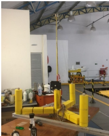
Fig. 3 Elastically and dynamically similar segmented backbone model
