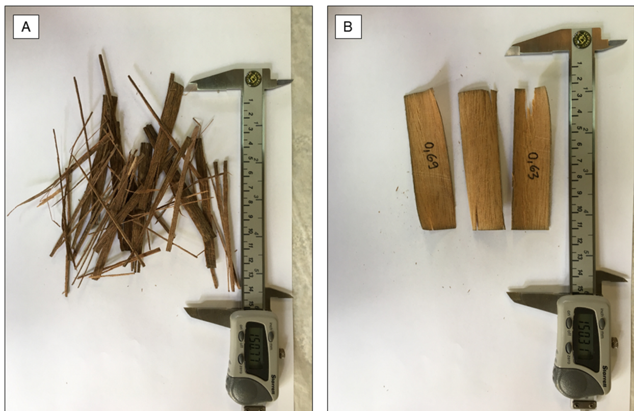
Figure 1. Wood strands before (A) and after (B) the blocks were soaked in hot water. (A) before heating in hot water, it was not possible to obtain entire strands, as they were brittle. (B) the quality of the strands obtained is superior to those made before the hot bath, as they are solid and have the appropriate geometry for the production of OSB panels. Note: The numbers in the strands in (B) represent the thickness.
