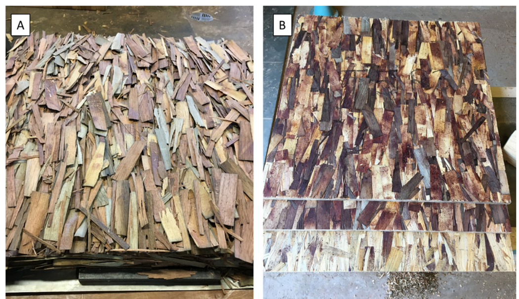
Figure 2. OSB panels from wood mixture. (A) Strands before pressing; (B) panel after hot pressing.
