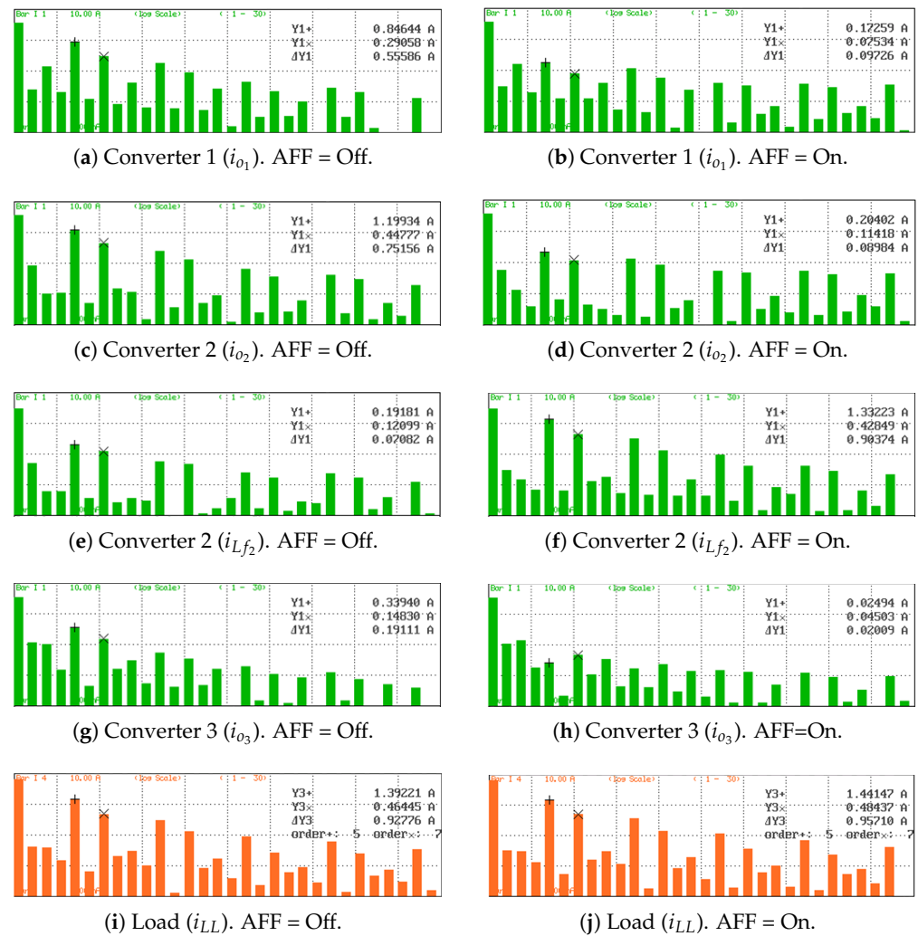
Figure 5. Current harmonic components in logarithmic scale for each power converter and the NLL.
