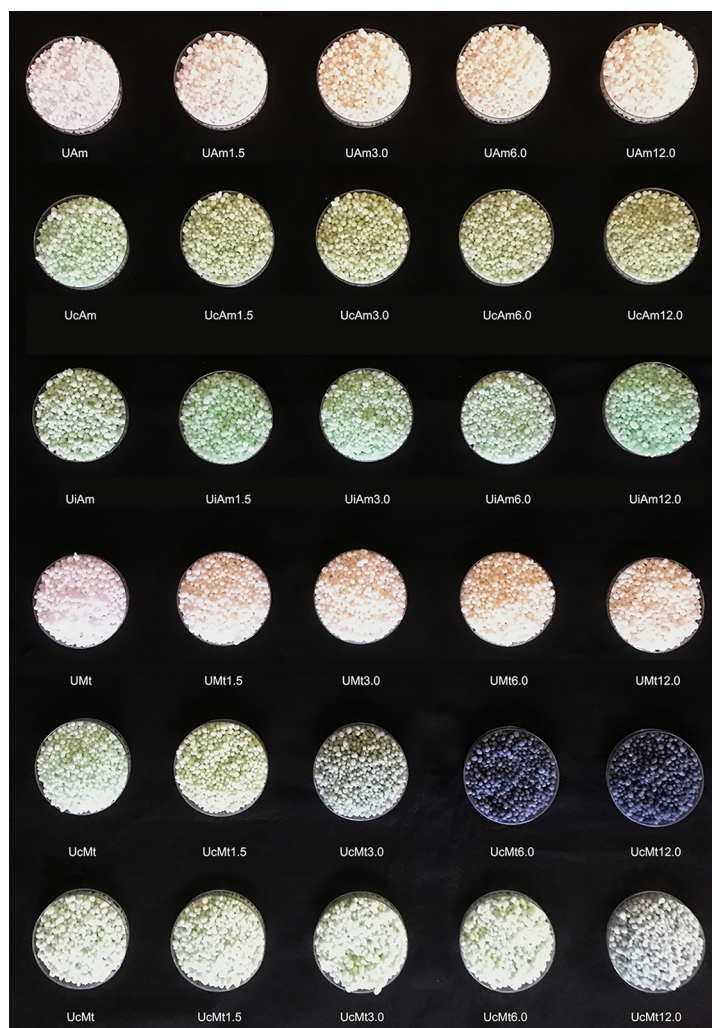
Figure 2 – Visual aspect of formulated nitrogen fertilizers formulated with or without N-(n-butyl) thiophosphoric triamide (NBPT) (U = Untreated urea; Uc = NBPT-coated urea; Ui = NBPT-incorporated urea), molybdenum (Mo) sources (Am = ammonium molybdate; Mt = molybdenum trioxide) and rates (0, 1.5, 3.0, 6.0, and 12.0 g kg -1 N).
