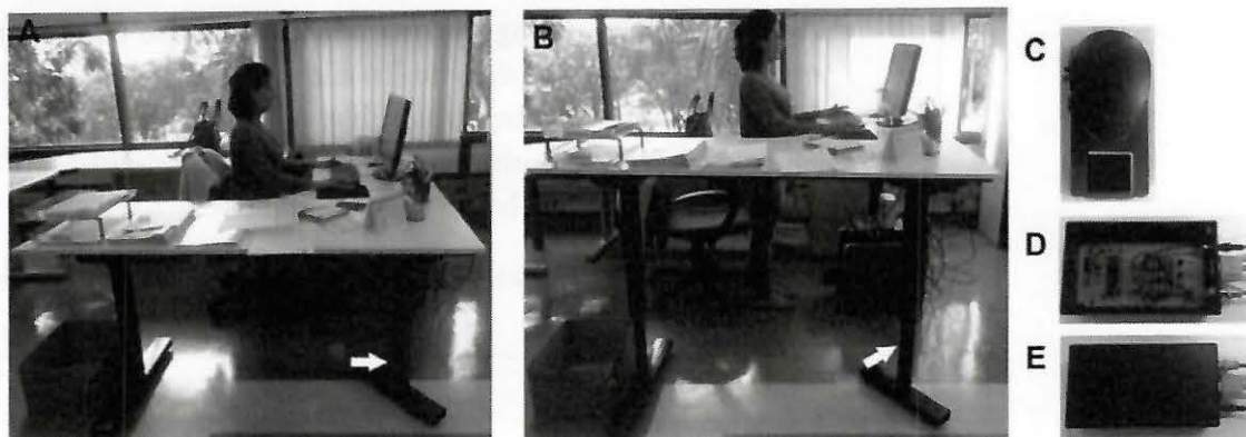
FIGURE 1 Electric lifting legs (arrows) of the sit–stand table (A and B); control box (C); and interface control board (D and E).
